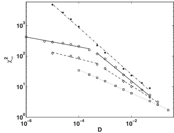
FIG. 5. Saturation value  $\chi_\infty^2$  over a wider range of diffusivity  $D$ , exhibiting different scaling over ranges of diffusivity. Parameter values shown are  $K=4.5$  (squares),  $K=5.5$  (diamonds),  $K=6$  (circles), and  $K=7$  (asterisks).
