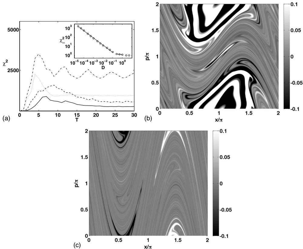
FIG. 2. (a)  $\chi^2(t)$  for mixed phase-space dynamics.  $K=2.1$  (solid),  $K=3.5$  (dashed),  $K=7$  (dotted), and  $K=8$  (dot-dashed).  $D=10^{-4}$  in each case. Note that all the curves go through the stages (a) rapid increase, (b) turnover, (c) decrease, and (d) steady state. Inset: saturation value of  $\chi^2$  as a function of  $D$  for  $K=7$ . (b) Persistent pattern for  $K=2.1$  and  $t=30$ . (c) Persistent pattern for  $K=7$  at  $t=30$ .
