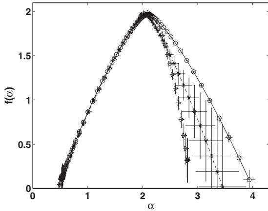
FIG. 4. Singularity spectrum with error bars for  $K=7$  (circles, solid line),  $K=9$  (triangles, dotted line), and  $K=12$  (crosses, dashed line). The values of  $\gamma$  are 0.8, 0.96, and 0.86, respectively.
