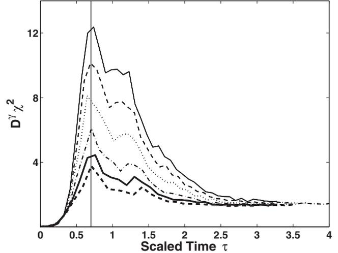
FIG. 3.  $\chi^2$  scaled by the  $D^{-\gamma}$  and time scaled by  $\ln 1/D$  plotted for  $K=2.1$  and values of  $D$  from  $5 \times 10^{-6}$ – $10^{-4}$ . The higher values of scaled  $\chi^2$  correspond to smaller  $D$ .
