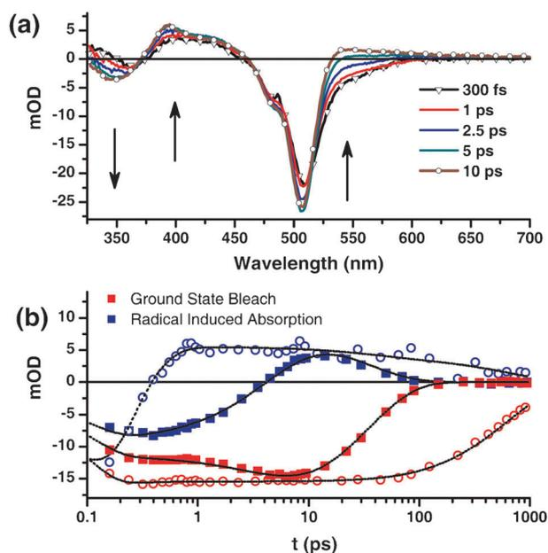
**Fig. 3** (a) Ultrafast transient absorption spectra of **1** after excitation at 509 nm in acetonitrile. (b) Time domain slices of the ground state bleach (red) and BODIPY radical absorption (blue) for dyad **1** (filled squares; bleach: 507 nm  $\times 0.55$ , induced absorption: 550 nm  $\times 2.5$ ) & **2** (open circles; bleach: 527 nm  $\times 2.5$ , induced absorption: 590 nm) with predicted traces based on a kinetic model (dashed black).
