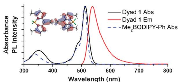
Fig. 2 Normalized absorption and emission spectra of dyad **1** and absorption spectrum of 3,5-Me<sub>2</sub>BODIPY–Ph in CH<sub>2</sub>Cl<sub>2</sub>. The LUMO surface of **1** is also shown.
